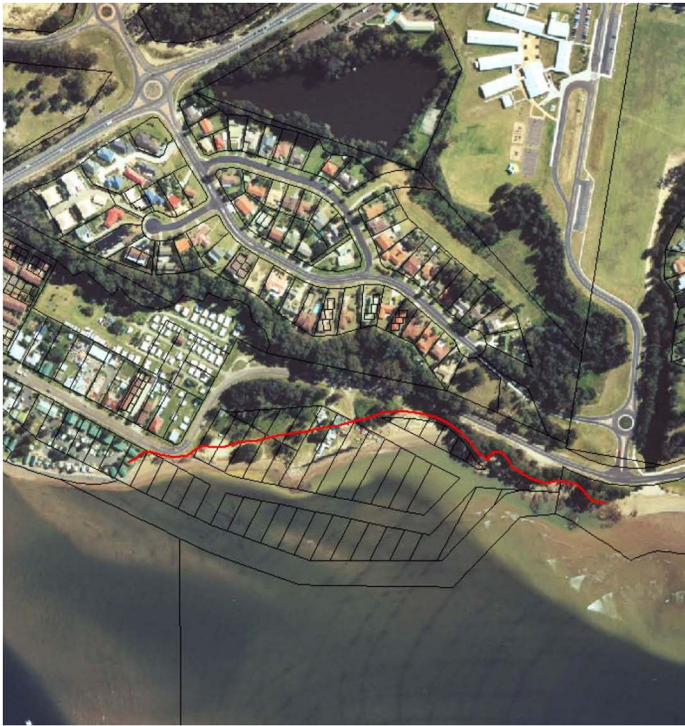
Figure 4: Wharf Road Precinct (2008) with overlay showing the position of the lots and the 100% line in red (Source: Draft Wharf Road Coastal Hazard Management Plan - BMT WBM Pty Ltd).
